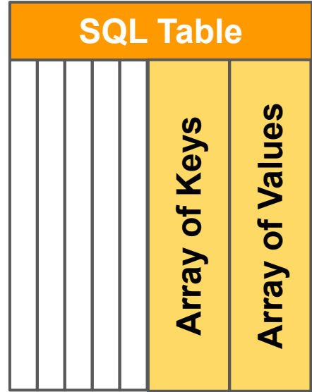
Arrays: Header values with key-value pairs
